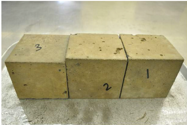
Penetrating (PS) treated concrete cube specimens
