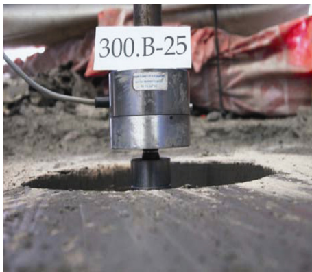
Fig. 6. Installation of bucket foundation ( D = 30 cm, embedment ratio 0.25)
