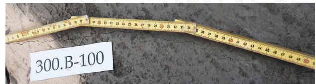
Fig. 11. Failure line in surrounding soil after testing 30 cm foundation
