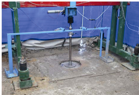
Fig. 9. Plate load test on 40 cm circular surface foundations
