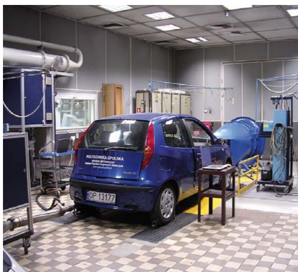
Fig. 1. Test car and bench test
